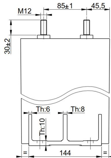
Max Torque M12: 25Nm
