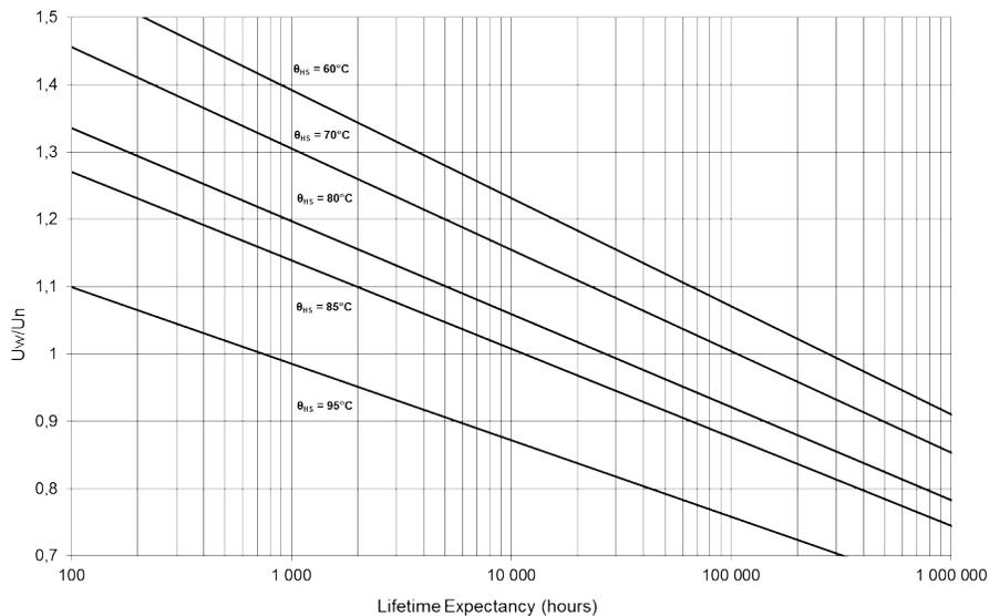
Expected lifetime at hot spot calculated at U<sub>w</sub>
