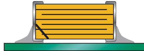
Type A: Angled crack between bottom of device to top of solder joint.
