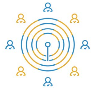
Active Antennas Eliminate nulls by "steering" the emission in real-time by using intelligent algorithms and flexible antenna structure
