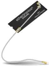
9000440 | Passive FPC Based Antenna (GPS)
